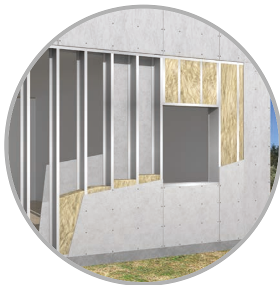
200mm wall 200mm insulation U-VALUE = 0.168 w/m 2 k
